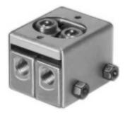
A push button operator or 2-position selector actuates both valves simultaneously. This arrangement is used for parallel control or 4-way valve functions. 2 position Square "D" selectors must have cam "A".
